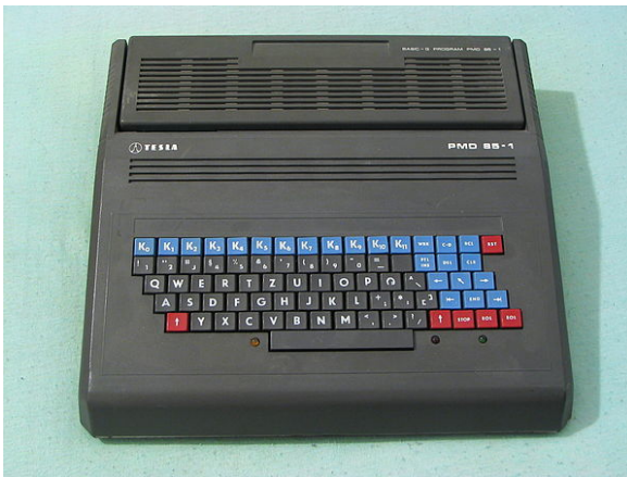
The 8-bit PMD 85 personal computer produced in 1985–1990 by the Tesla company in the former socialist Czechoslovakia. This computer was produced locally (in Piešťany) due to a lack of foreign currency with which to buy systems from the West.
