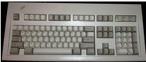
A “Model M” IBM computer keyboard from the early 1980s. Commonly called the “Clicky Keyboard” due to its buckling spring key design, which gives the keyboard its iconic ‘Click’ sound with each keystroke.
